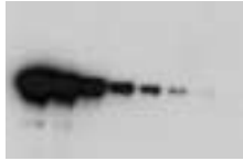
Figure 3: Detection of low picogram concentrations of Mouse IgG using LumiGLO Reserve at the optimized conjugate dilution. Non-reduced Mouse IgG was transferred to the blots at 500 pg, 250, 125, 62.5, 31.25, 15.6, 7.8, 3.9 pg. Sample was detected using anti-mouse HRP antibody (1:10,000) and LumiGLO Reserve and exposed to film for 5 minutes.
